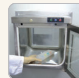
③ Secure electronic airlock for a sample transfer
